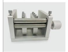
Automatic plate feeder for serial marking and cutting;
