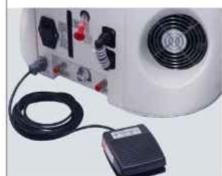
Foot pedal offers hands-free control for operating laser machines, providing convenience and flexibility.
